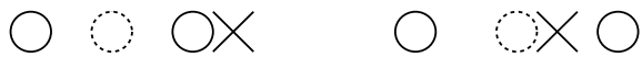
Figure 6: Circles: two inaccurate detections, one from the current frame and one shifted from the last frame. Dotted circle: Average position of the two circles. Cross: ground truth. Only in the right example the dotted circle is closer to the ground truth than the average distance of the two normal circles to the ground truth. As the position variations of the eye detector is mostly like on the left (one sided error) there is no big benefit for our information fusion approach in average pixel location error. However, the dotted circle is less noisy in position than the original circles which supports prediction (see text).
